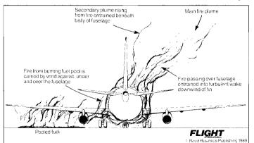
rate, but overlapping, phases, involving fundamentally different fire mechanisms. While the aircraft was moving at speed down the runway, fuel became entrained into a strong turbulent wake generated by the extended thrust-reverser buckets, and burned vigorously as a "dynamic fire plume". As the aircraft decelerated and the turbulent wake decayed, the fire transitioned into a quasi-static fire burning above the pool of fuel trailing behind the aircraft.
